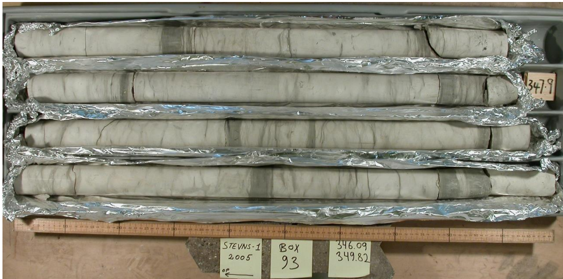
Figure 6. Part of Boesdal Member in Stevns-1 core, with alternating chalk, marly chalk and marl (dark grey layers).
