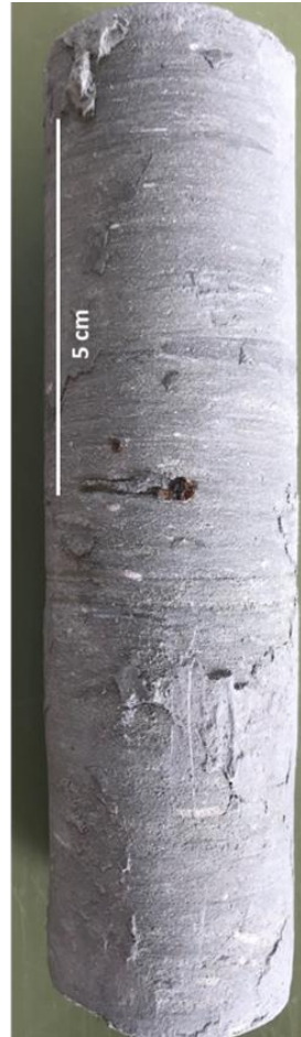
Facies 32. Grey, laminated, calcareous mudstone, Upper Cretaceous. Core 7, 1125–1135'.
