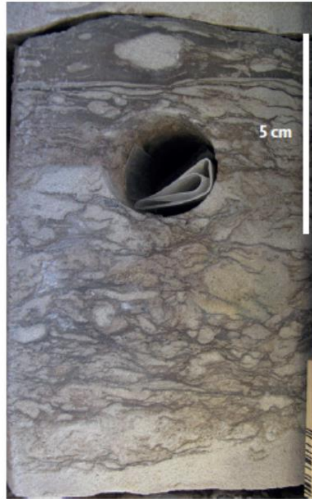
Very fine grained sandstone, primary sedimentary structures obliterated due to bioturbation. Stenlille-4, core 2, box 6.
