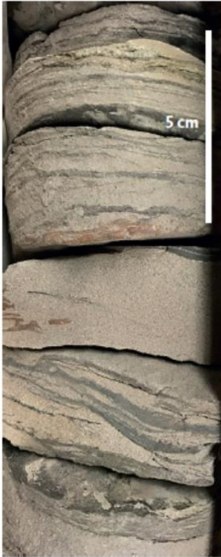
Fine grained, heterolithic sandstone. Gassum Fm. Flyvbjerg-1, core 6, box 4, 1316 m
