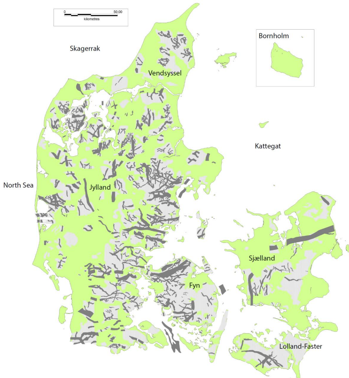
Figure 2.7. Mapped buried valleys in Denmark shown with dark-grey polygons. The light grey colour indicates areas mapped using the Transient ElectroMagnetic method (TEM). Modified from Sandersen & Jørgensen (2017).
