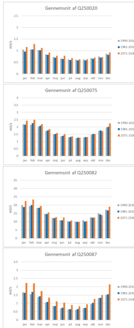
Figur A6-3: The figure shows graphs of the simulated mean mounthly discharge, at Q250020(Holtum å), Q250075(Hover å), Q250082(Skjern å) and Q250087(Venner å), in a 30-year period for the four climate models in Ringkøbing catchment . The grey colums represent the historical model run in the period 1989-2018, where the blue colums represent the simulated discharge for the four climate models in the period 1981-2010, whereas the orange colums represent the simulated discharge for the four climate models in the period 2071-2100(RCP 8.5)/2041-2070(RCP 4.5).
