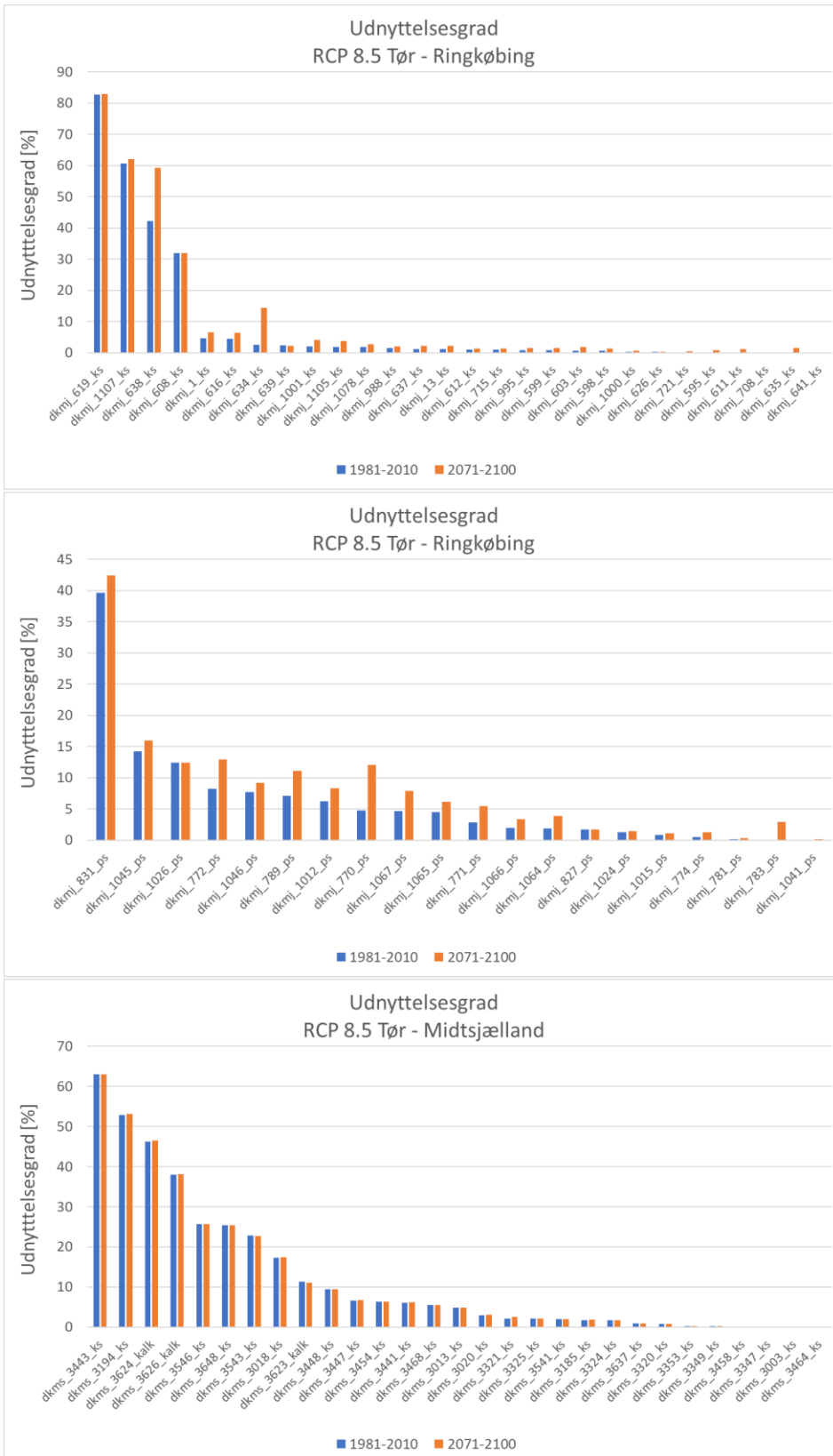
Figure A47-6 Graphs showing the the difference of abstraction versus groundwater recharge for groundwater bodies for future and present climate in the Ringkøbing fjord catchment(upper and center graph) and Midt-Zealand(Lower graph) in the RCP 8.5 dry climate model.
