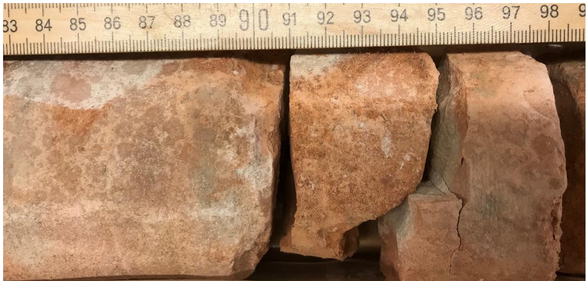
Figure 14. Drill core from the Rødby-1 well demonstrates the red, sandy, calcareous siltstone of the Rødby Formation, upper part of the Lower Cretaceous.
