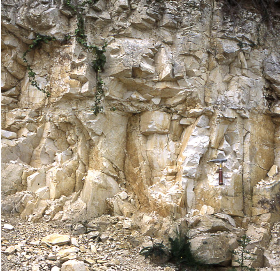
Figure 34. Danian limestone intersected by horizontal and vertical fractures, Amager (hammer for scale).
