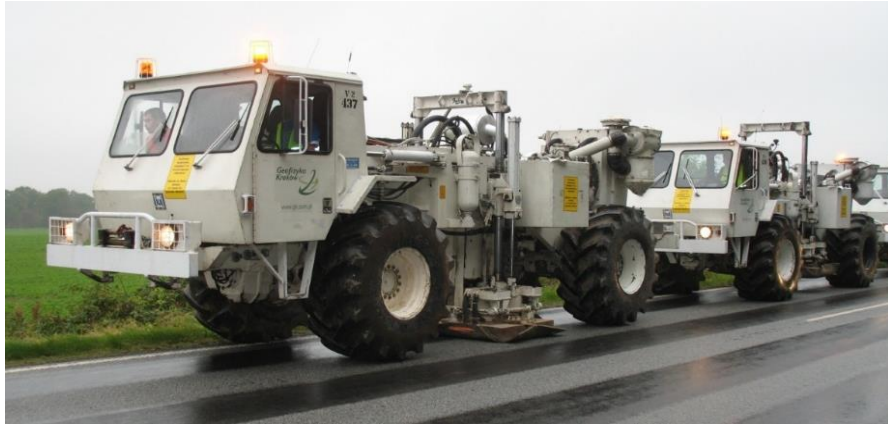
Figure 4. Vibrator vehicles at work. By using multiple vehicles that use their vibrators synchronously, the sound waves are amplified to the subsurface. This provides a better seismic signal and thus a more detailed picture of the subsurface.
