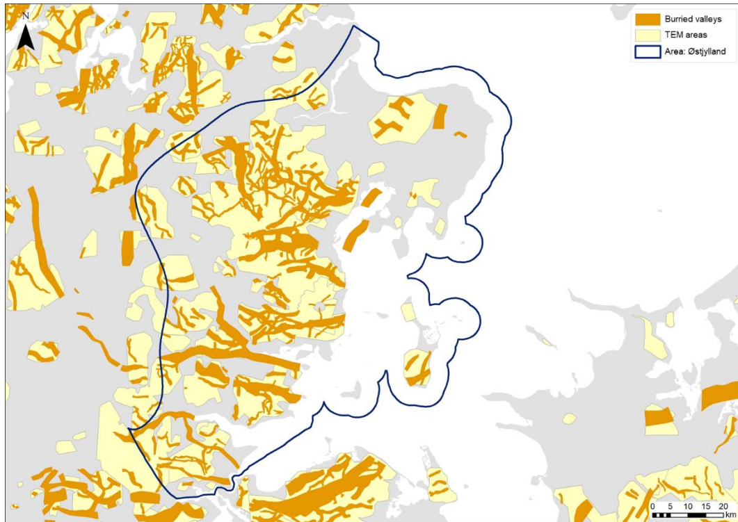
Figure 6.57. Mapped buried Quaternary valleys (orange) and the coverage of TEM data used for mapping, Østjylland area.
