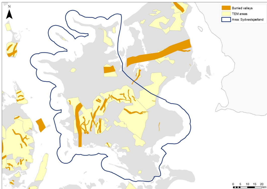
Figure 6.128. Mapped buried Quaternary valleys (orange) and the coverage of TEM data used for mapping, Sydvestsjælland area.
