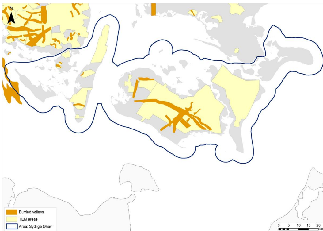
Figure 6.114. Mapped buried Quaternary valleys (orange) and the coverage of TEM data used for mapping, Sydlig Øhav area. Most of the area is covered by TEM surveys and in large parts of the area buried valleys have not been identified.
