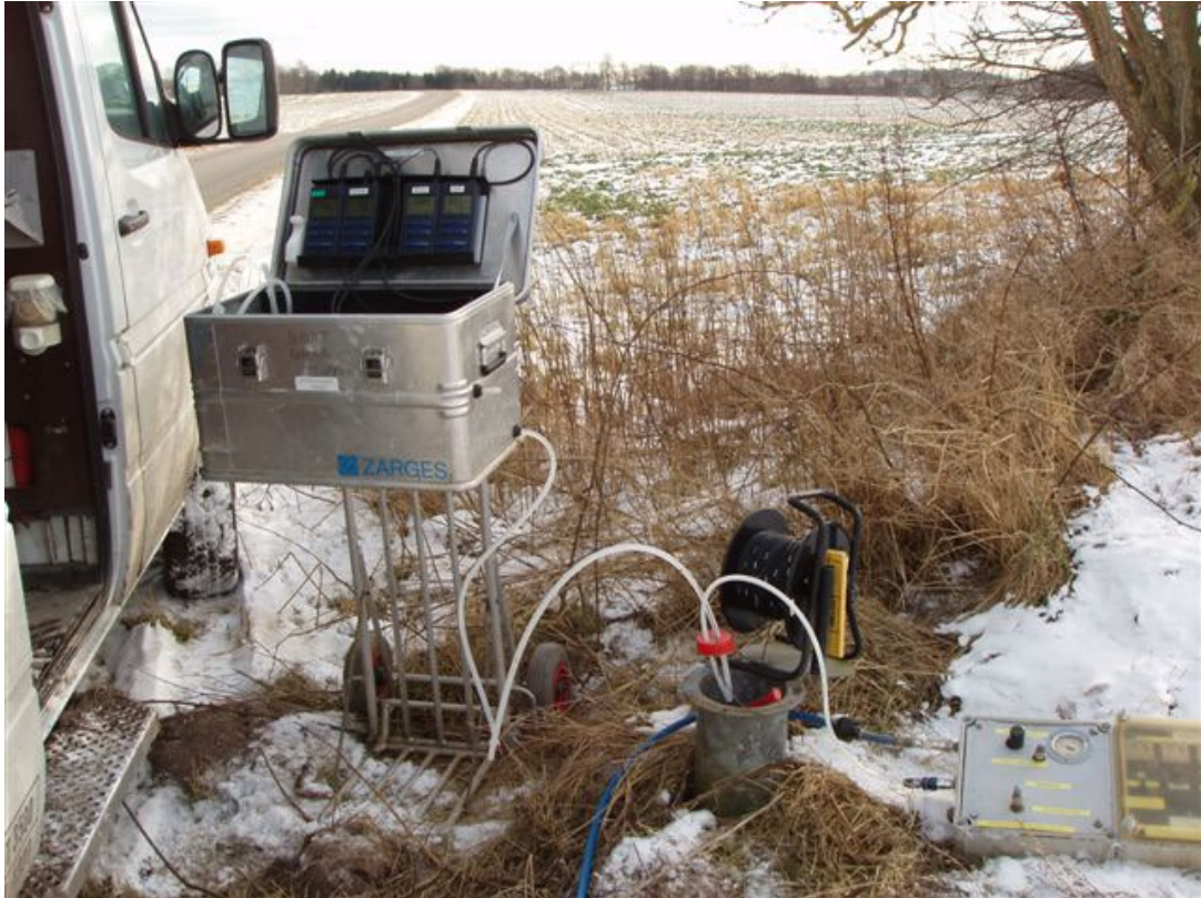
Figure 5. Example arrangement of equipment for field measurements with a montejus pump. Note the control box placed on the ground used to control the sampling process.
