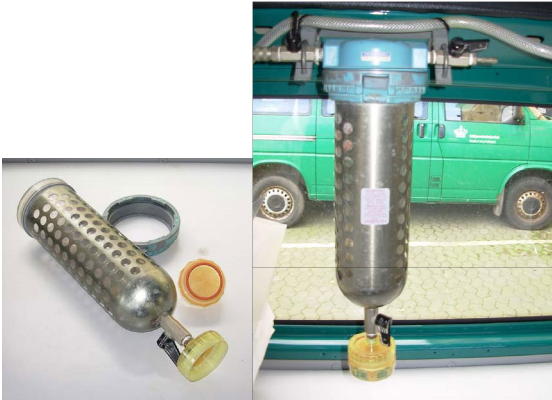
Figure 3. Pressure filtration equipment from LOOP is also used in wells with insufficient pumping pressure. The figure shows the filter casing and filter holder as well as the field vehicle installation with gas for pressure filtration mounted.
