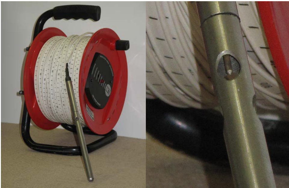
Figure 3. Manual water level meter. This meter emits a signal when an electrical current flows between the two electrodes of the meter. This occurs when water conducts electricity between the electrodes, see the image on the right. Note: Erroneous readings may arise if the water causing electricity to flow is due to condensation from the well casing. Groundwater with a low conductivity will create a weaker circuit which weakens the signal produced.
