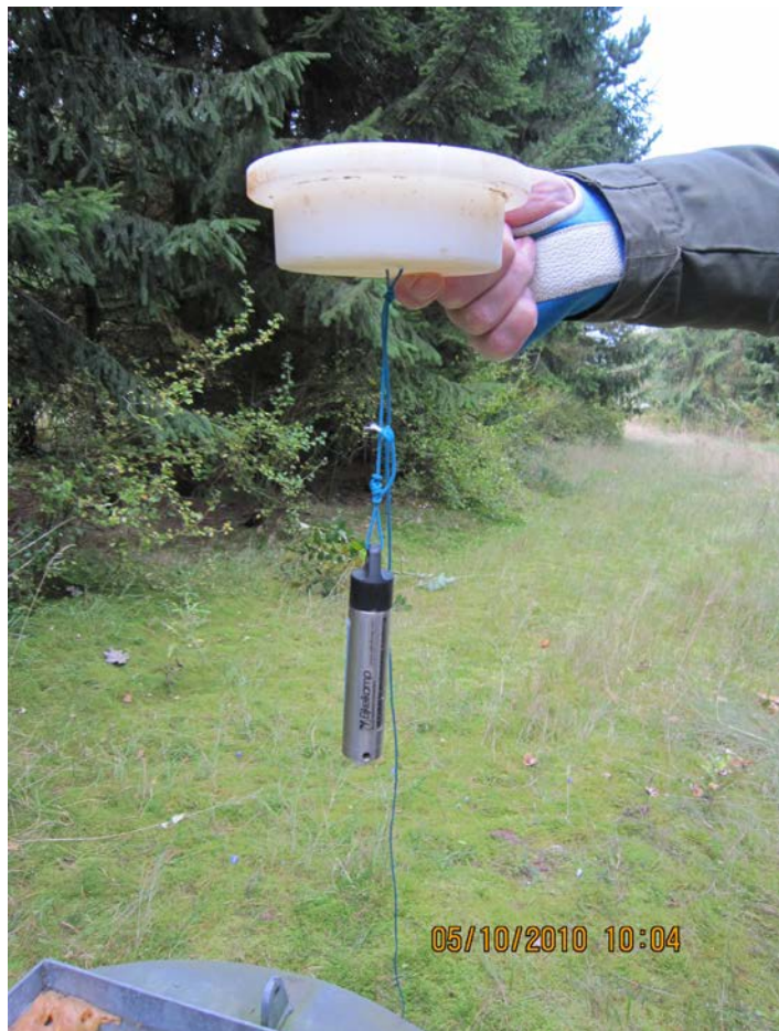
Figure 5. Barodiver suspended at the top of a well above the water table with a view to measuring air pressure. It should be suspended a minimum of 3 meters below the surface to ensure frost-free conditions. If the logger is mounted as described, it is important to remember to make a hole in the well lid to enable pressure equalisation between the well and the atmosphere. To minimize the influence from wind-borne contamination and precipitation, the hole should be as small as possible and be placed keeping the contamination risk in mind.
