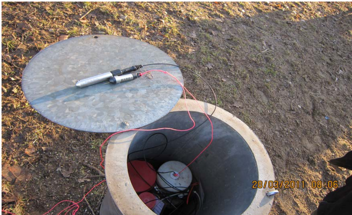
Figure 4. Two different types of pressure transducers before mounting in a well. A larger older version and the smaller, newer version.
