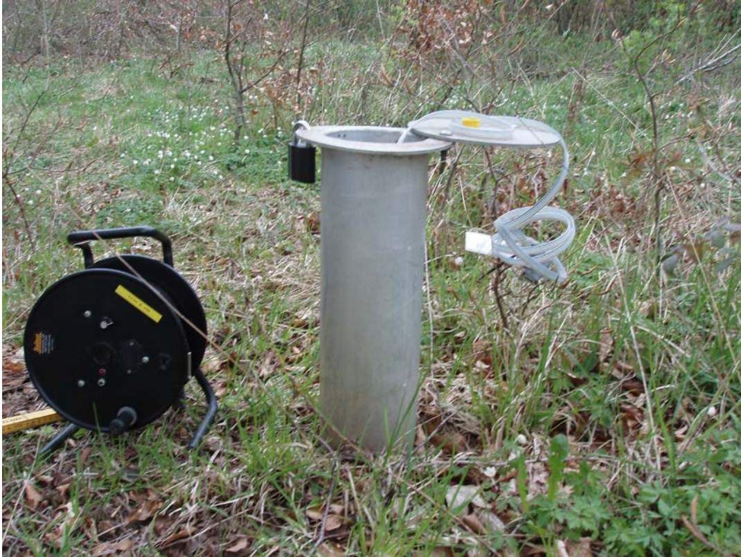
Figure 2. Hand-held water level meter and folding ruler at well. Note how the hand-held meter is easily identifiable owing to the yellow "dymo marking".
